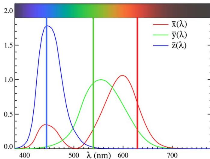
Figure 2: Eye response diagram highlighting the responses to a representative selection of red, green and blue primaries.
