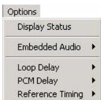
To see the results on an OmniTek LAB, display the Delay Measurement window – for example by clicking on its icon in the main (Window) toolbar and use its Options menu to set it to display the appropriate Loop delay. The total propagation delay through the external equipment is calculated and displayed as illustrated below.
