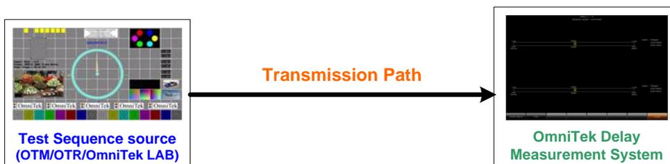
Figure 1: Basic setup for Lip-Sync Delay measurement.
