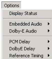
To display the Lip-Sync Delay affecting PCM embedded audio, use the **PCM Delay** option in associated Options menu to select PCM Relative Delay and use the **Embedded Audio** option in the same menu to select the channel on which the test is to be run.
